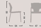
SR 10-SR11 Sedia 4 gambe cromata senza braccioli. Four legs chromed chair without armrests.
